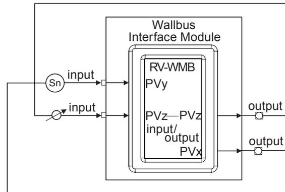
This can be seen in the diagram where PVx is an output from the RV-WMB which is connected to a sensor module in the strategy. The sensor's output is then sent back to the RV-WMB for display (PVy). This enables the strategy to change the value before display (e.g. apply an offset).
